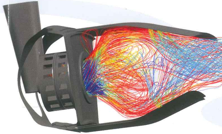
Full Annular combustor - A. Andreini
